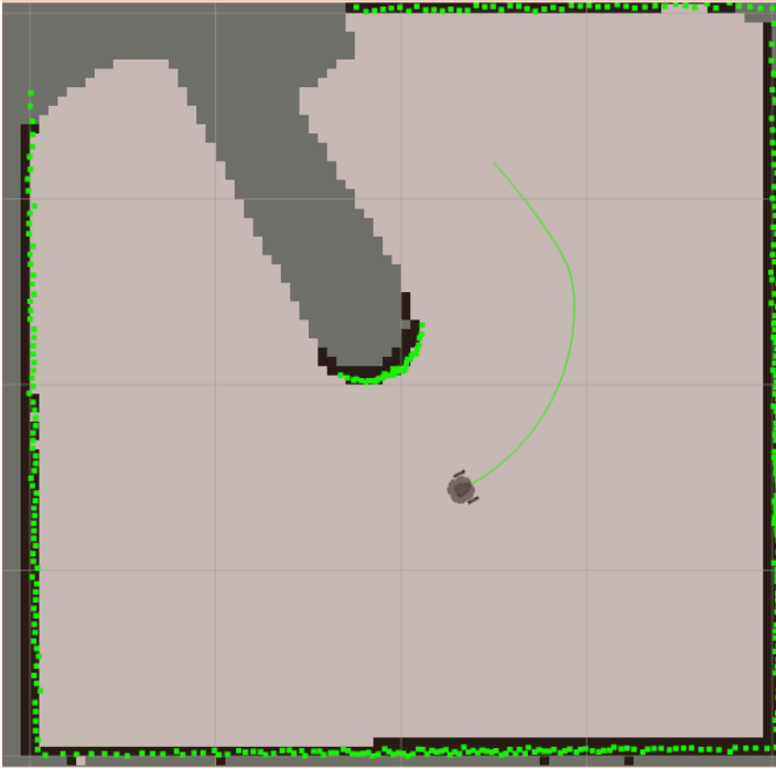
Figure 11: Screenshot of rviz with a trajectory planned to a 2D nav goal using RRT.
